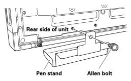
Tighten the Allen bolt using an Allen wrench (width across flats of 6 mm).
